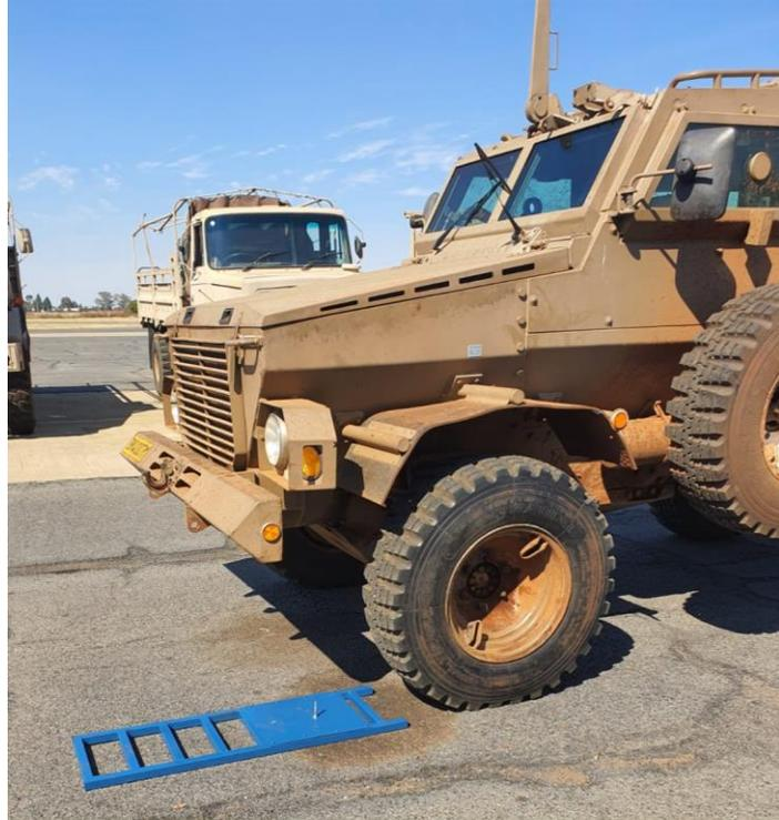
Liquid Seal used to keep a Mamba armoured personnel carrier moving after a puncture.
